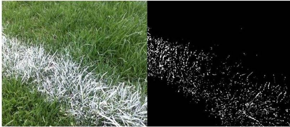
Figure 14: (a) Raw Image from Camera, (b) Filtered Image with 5% White Detected
